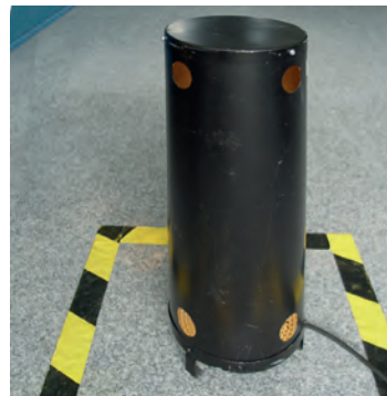
Abb. A50 Kühllastsimulator (IBP)
