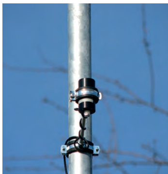
Abb. A9 Pyranometer vertikal (THN-AR)
