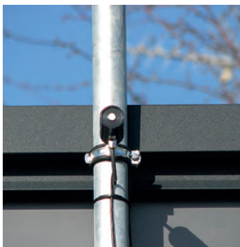
Abb. A8 Pyranometer horizontal (THN-AR)
